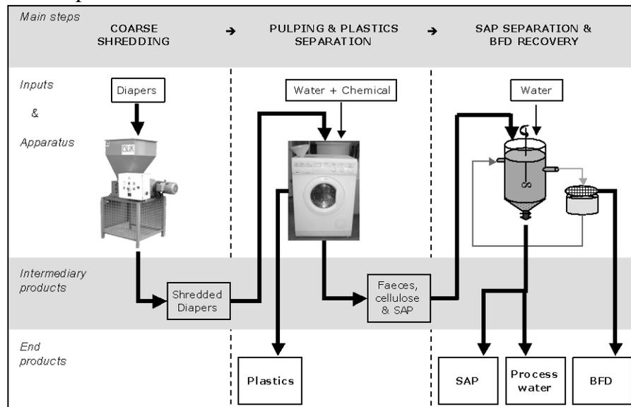
Figure 1: Lab-scale process used for the separation of the constituents of used disposable diapers (SAP: Super Absorbent Polymer; BFD: Biodegradable Fraction of Diapers)
