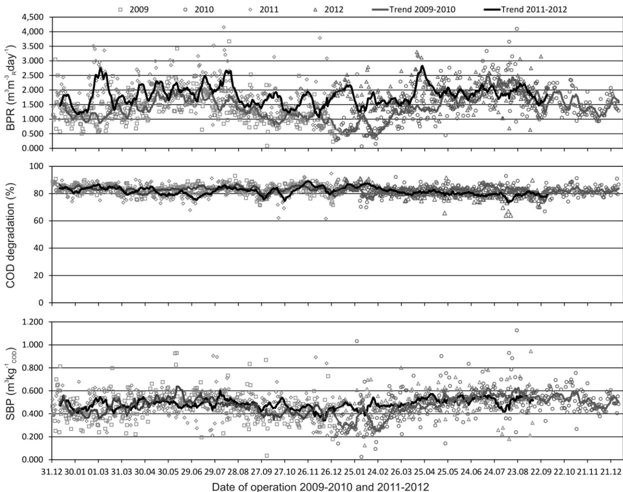
**Figure 2.** Results of full scale operation: Biogas production rate (BPR), COD degradation and Specific biogas productivity (SBP).
