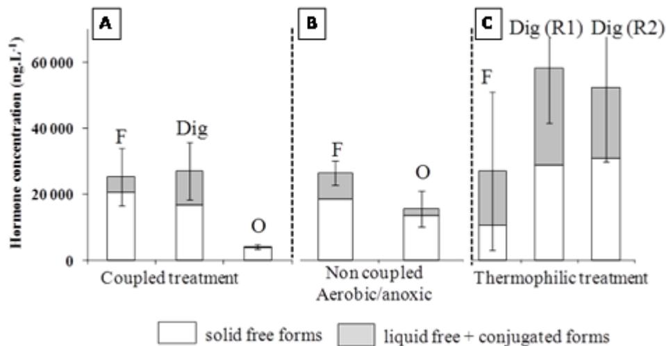
**Figure 1.** Fate of steroid hormones (A, B, C) during manure treatment. Concentrations in each compartment of the studied systems: Feed (F), Digester (Dig) and outlet (O) of the three treatment processes.
