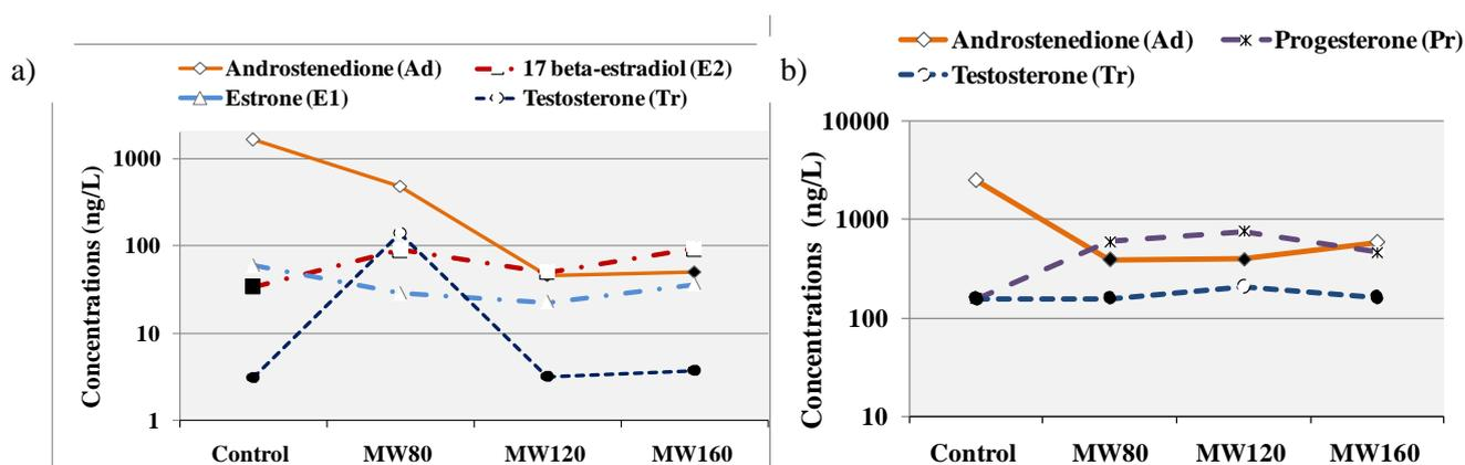
**Figure 1.** Effect of microwave (MW) on hormone concentrations in the a) soluble (supernatant) phase and b) total (sludge) phase of the influent (Control: un-pretreated; 80, 120 and 160: MW pretreatment temperatures in °C; single data point concentrations; black filled data points represents concentrations below reporting limit).
