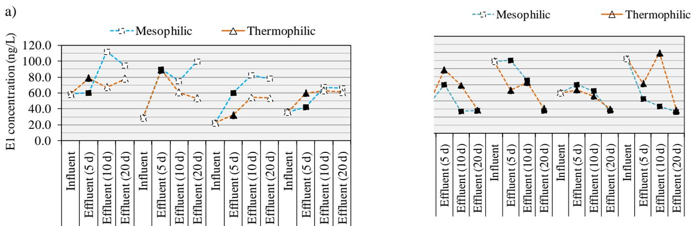
**Figure 2.** Concentrations of a) estrone (E1) and b) 17 $\beta$ -estradiol (E2) in soluble phases of the influent and effluents at different solid retention times (SRTs) (Control: un-pretreated; 80, 120 and 160 are ultimate microwave pretreatment temperatures in °C unit; black filled data points were below reporting limit (RL). RL varied as E1: 32 – 90 ng/L, E2: 26.2 – 90 ng/L).
