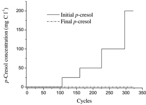
**Figure 1.** *p*-Cresol consumption in a nitrifying sequential batch reactor.
