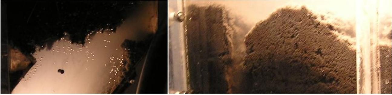
**Figure 3.** Anaerobic sludge clogging within the lamella separator because of low flow velocities (left); accumulating sludge within the integrated clarifier because of turbulence eddies underneath which prevent sedimentation
