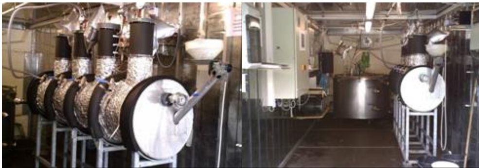
Figure 1. Pilot plant. Left: Horizontal digester with feeding screw and gas domes. Right: Storage tank for inoculation of the plug flow fermenter.
