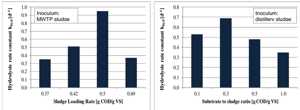
**Figure 2.** Influence of SLR on hydrolytic activity for MWTP-sludge (left) and distillery sludge (right)
