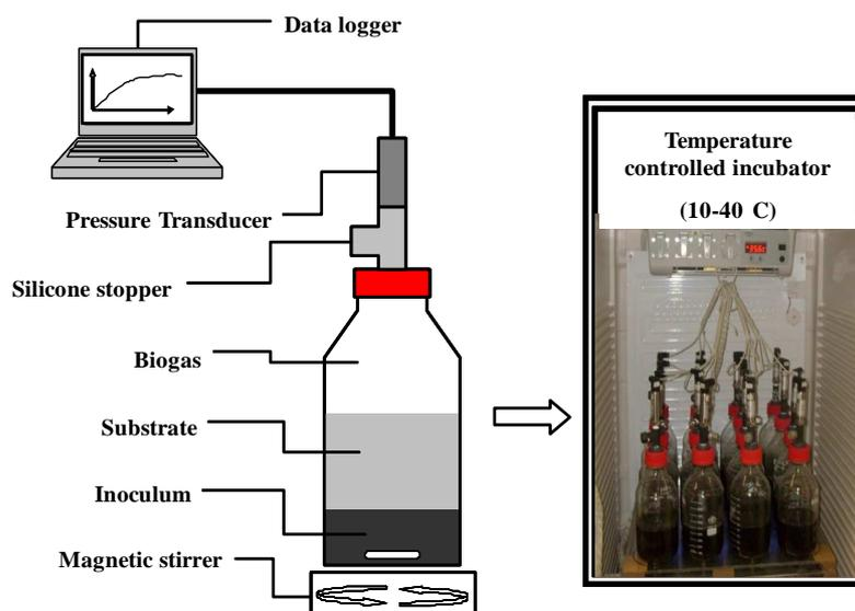
**Figure 1.** Anaerobic batch test apparatus in accordance with DIN EN ISO 11734
