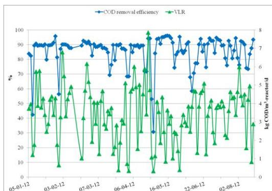
Figure 4: Results of COD removal efficiency and VLR at the ice cream factory.
