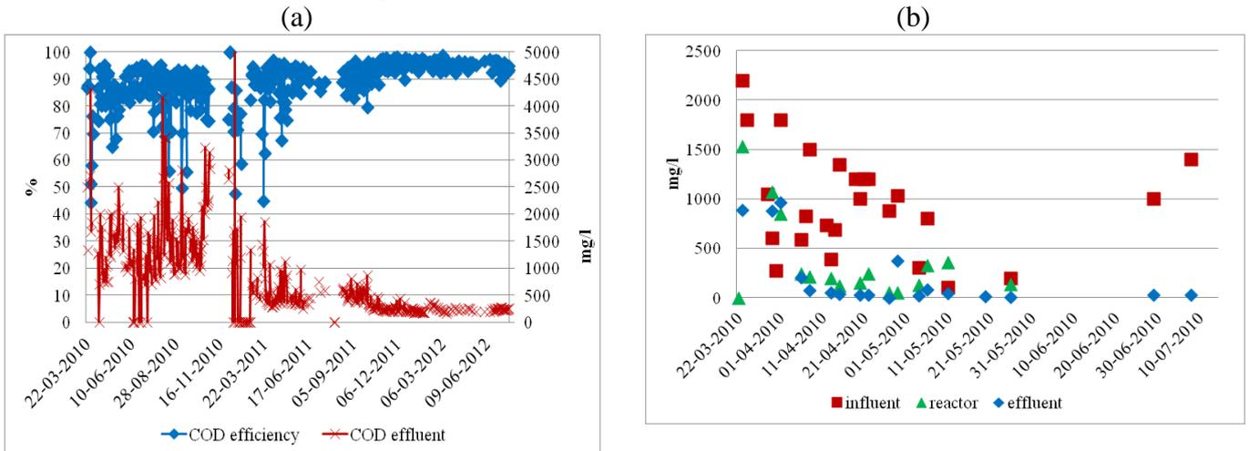
Figure 3: (a) COD removal efficiency and COD effluent. b) fat concentrations in the influent, sludge and effluent of the AFR at the tank cleaning company.
