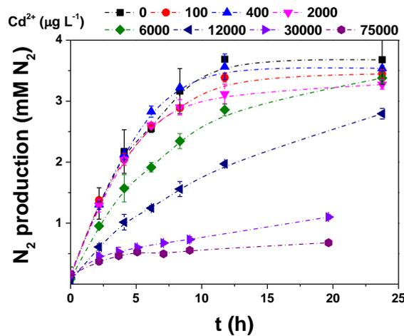
**Figure 2.** Effect of Cd<sup>2+</sup> on nitrogen production by anammox granules. Error lines represents standard deviations from duplicates.
