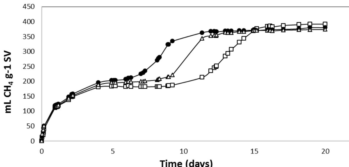
**Figure 1.** Methane yields obtained through BMP test for OMSW without pre-treatment ( $\Delta$ ) and OMSW pre-treated at 120°C (180 min) ( $\square$ ) and at 180°C (180min) ( $\bullet$ ).
