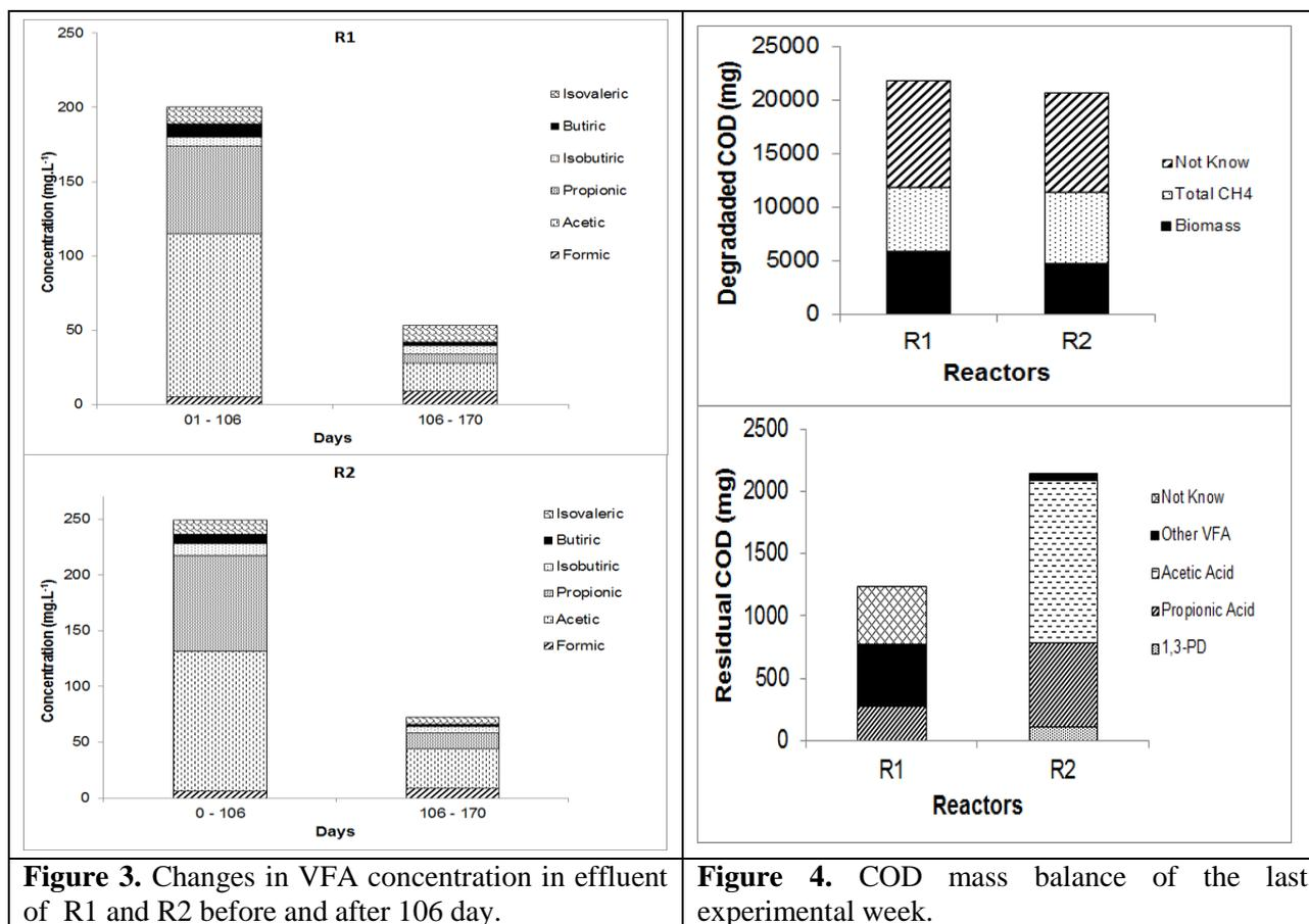
**Figure 3.** Changes in VFA concentration in effluent of R1 and R2 before and after 106 day.
