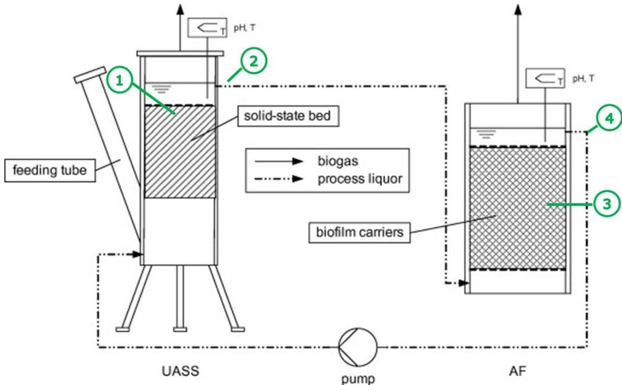
**Figure 1.** Overview about the experimental setup (UASS, up-flow anaerobic solid-state reactor; AF, anaerobic filter) and the collected samples (1 digestate; 2 effluent UASS; 3 biofilm carrier; 4 effluent AF) (modified after Pohl et al. 2012).
