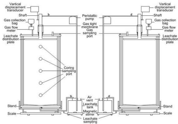
**Figure 1.** Schematic of simulators #2 (right) and #3 (left).
