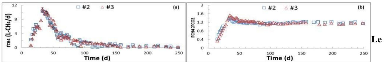
**Figure 2.** Methane generation rate (a) and ratio between  $r_{CH_4}$  and  $r_{CO_2}$  (b) for simulators #2 (blue) and #3 (red).
