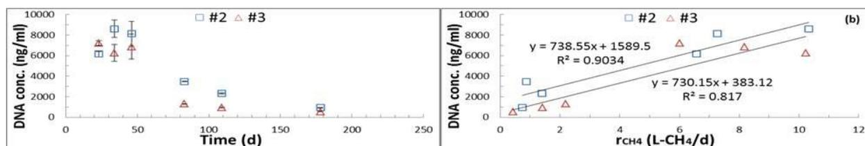
**Figure 4.** Biomass concentrations in leachate of simulators #2 (blue) and #3 (red) (a) and correlations with  $r_{CH_4}$  (b).
