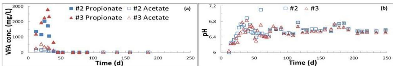
**Figure 3.** Concentrations of VFAs (a) and pH (b) of leachate collected from simulators #2 (blue) and #3 (red).
