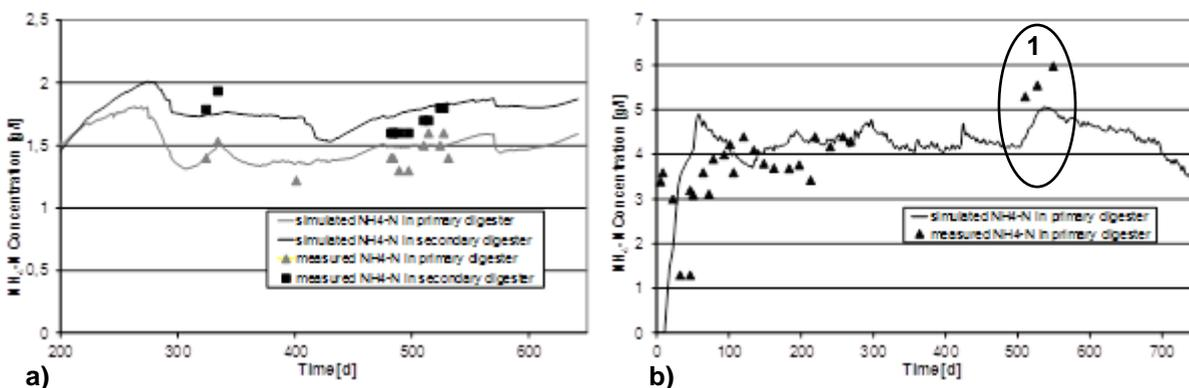
**Figure 2.** Measured and simulated  $\text{NH}_4\text{-N}$  concentrations for the digesters, a) biogas plant *Lelbach*, b) biogas plant *Wambeln*
