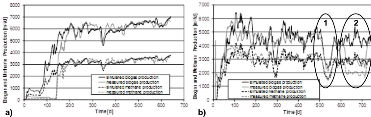
**Figure 1.** Measured and simulated methane and biogas production, a) biogas plant *Lelbach*, b) biogas plant *Wambeln*
