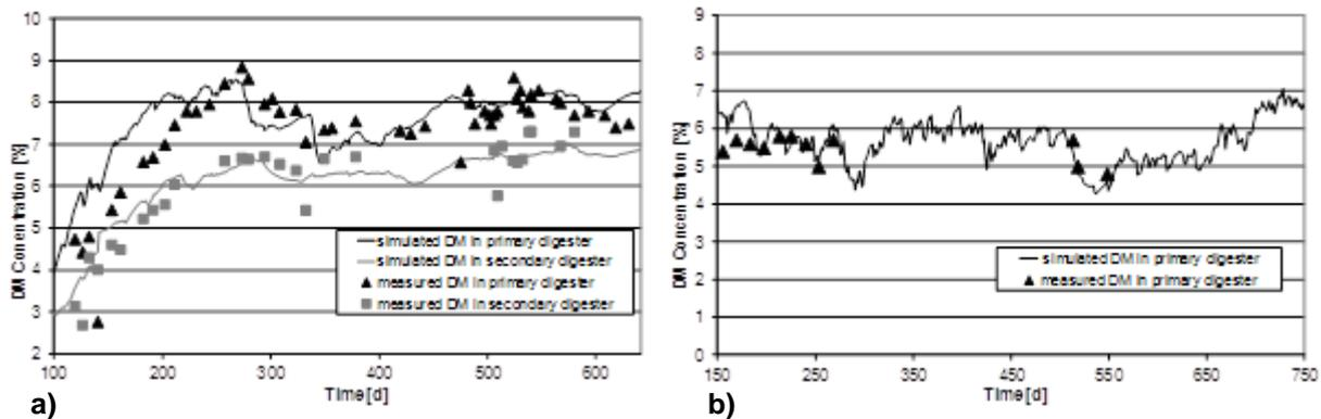
**Figure 3.** Measured and simulated DM concentrations for the digesters, a) biogas plant *Lebach*, b) biogas plant *Wambeln*
